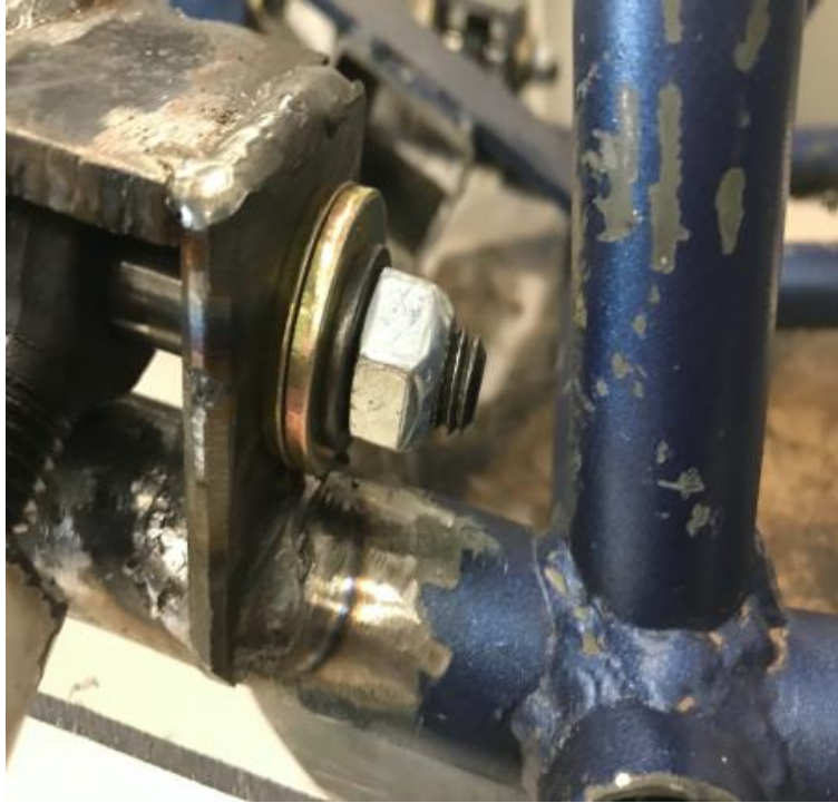
Figure 1: Steel welded on the front suspension
