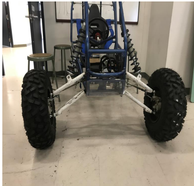
Figure 2: Final design for front suspension
